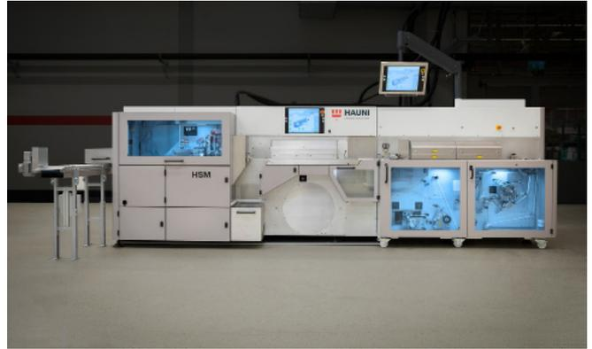
The Hauni Straw Maker allows you to produce visually appealing, high-quality, biodegradable straws. They have a smooth surface without overlapping paper, are food-safe and contain only minimal amounts of adhesive. Thanks to the market-proven, high-tech HSM process, you only need one type of paper to produce the straws, thereby saving material:
